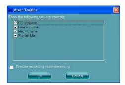
ALC888 allows you to record the CD, Line, Mic and Stereo Mix channels simultaneously, frees you from mixing efforts. At any given period, you may choose 1 of the following 4 channels to record.
